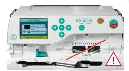
CAUTION! Ensure that the line guide is straight and avoid sagging/bending, otherwise the line may be damaged and could cause incorrect dosing.
