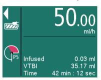
The set pressure level is shown with a P (for pressure) and a number. In addition, a red area shows how quickly the set pressure alarm limit will be reached. The "manometer" display shows the current pressure in the system. The lower the set pressure alarm limit level is, the larger the red area is, the quicker this limit is reached and a pressure alarm triggered.
