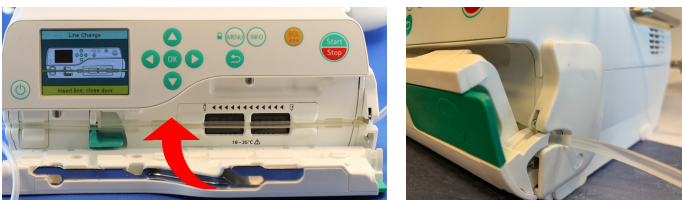
Fig. 7 - 7 Second clamp opened (right)
