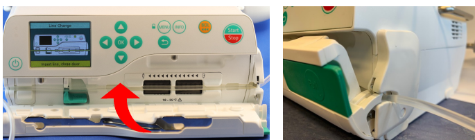
Fig. 4 - 7 Second clamp opened (right)
